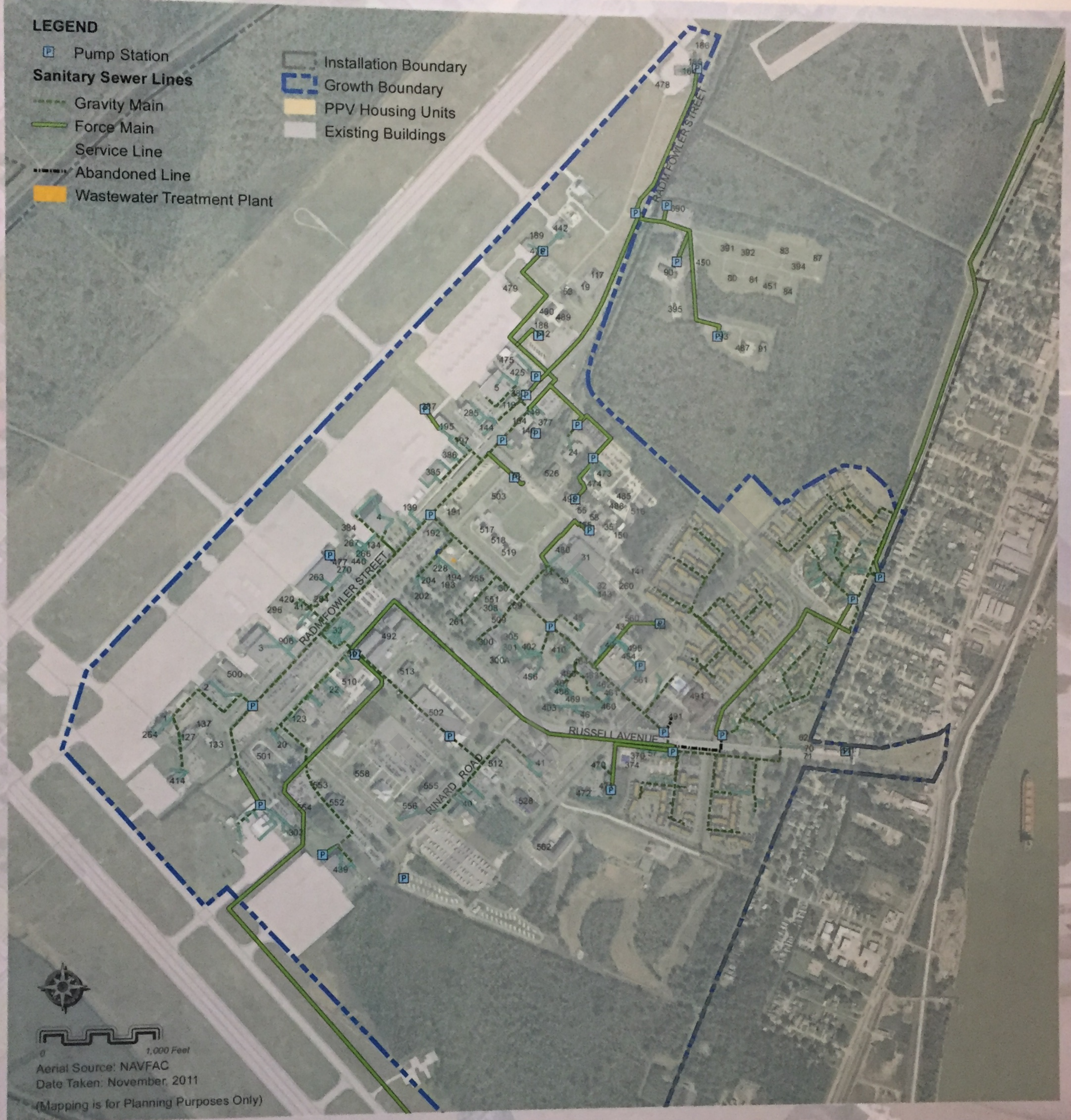
EXHIBIT 2.4, SANITARY SEWER NAVAL AIR STATION JOINT RESERVE BASE NEW ORLEANS MASTER PLAN MAP BOOK
