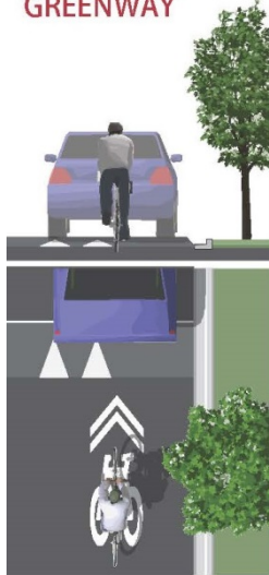
Shared Travel Lane with pavement markings and traffic calming
