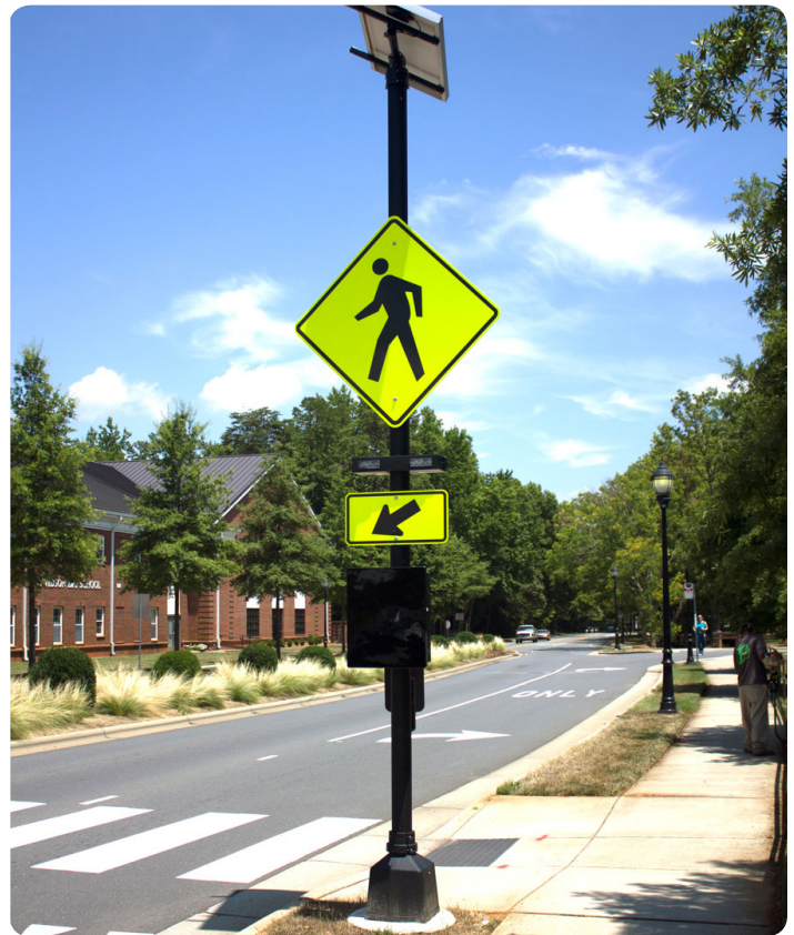
Figure 7 - Rapid Flash Beacon
