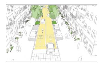
Raised Intersections, Changes in Road Texture Can use grooved asphalt, colored paving stones, brick, or for the ultimate effectiveness, cobblestones.
