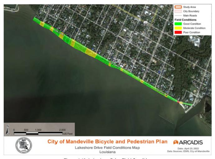
Figure 4-13: Lakeshore Drive Field Conditions
